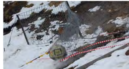
Figure 4. Full scale impact test, type 2 (Fulde, 2013)
