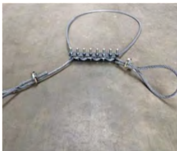
Figure 6. Friction dissipator (Dugelas, 2020)
