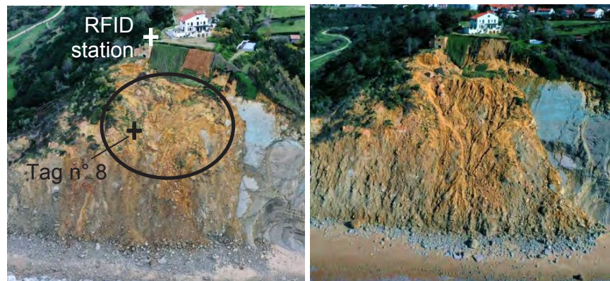
Figure 2: Villa Itxas Gañana landslide (left) on 15/12/2022 and (right) on 20/01/2023, highlighting the transformations caused by the exceptional acceleration of January 17 th . The site was equipped with an RFID station (white cross), 30 tags deployed over the landslide (black circle, and black cross for the tag n° 8)
