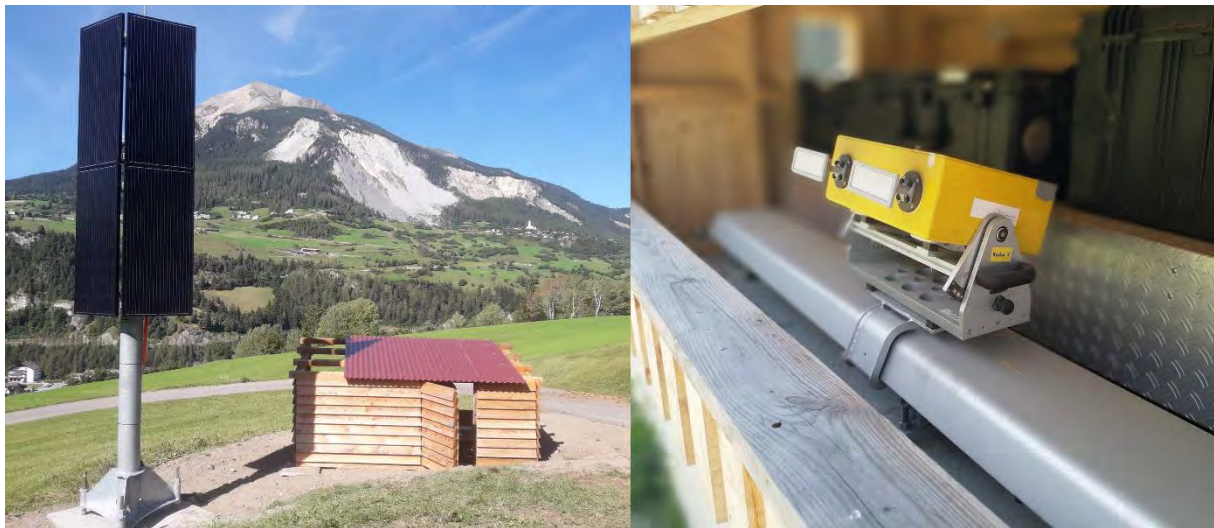
Figure 1. Left: location of the interferometric radar with the solar panels and the hut (under construction). Right: radar head moving on the system's rail with protection cases containing the batteries, the fuel cell and the transmission unit.
