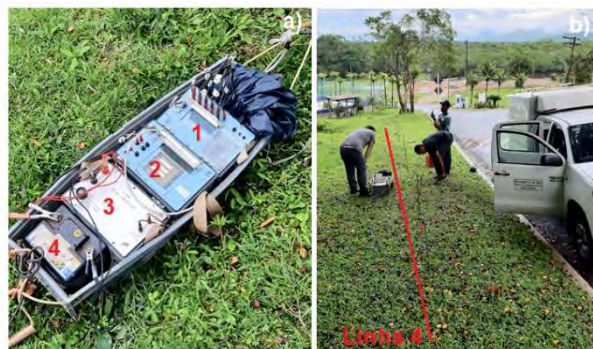
Figure 1. a) Rho/IP System used in electrical propagation, 1 (receiver), 2 (transmitter), 3 (DC/DC converter), 4 (battery). b) Data acquisition along Line 4
