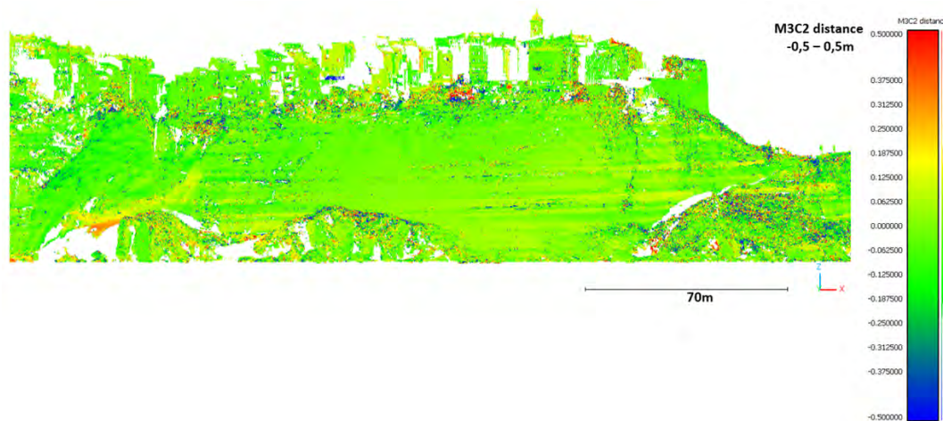
Figure 3. Cloud to cloud comparison (diachronic comparison 2018-2023). The main negative distances are due to coastal erosion and variations in vegetation.
