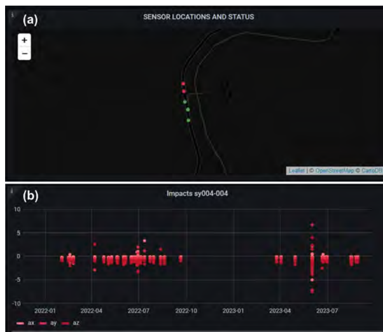
Figure 3. Dashboard via Grafana. Besides the exact location (a) of each sensor, the data can be observed and qualitatively analysed in several plots (b).
