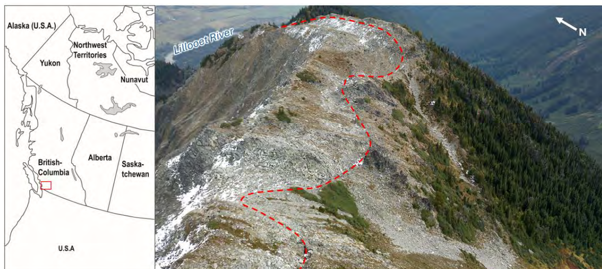
Figure 1. Location map and overview of potential rock avalanche source 1. Dashed red line highlights main down dropped block.
