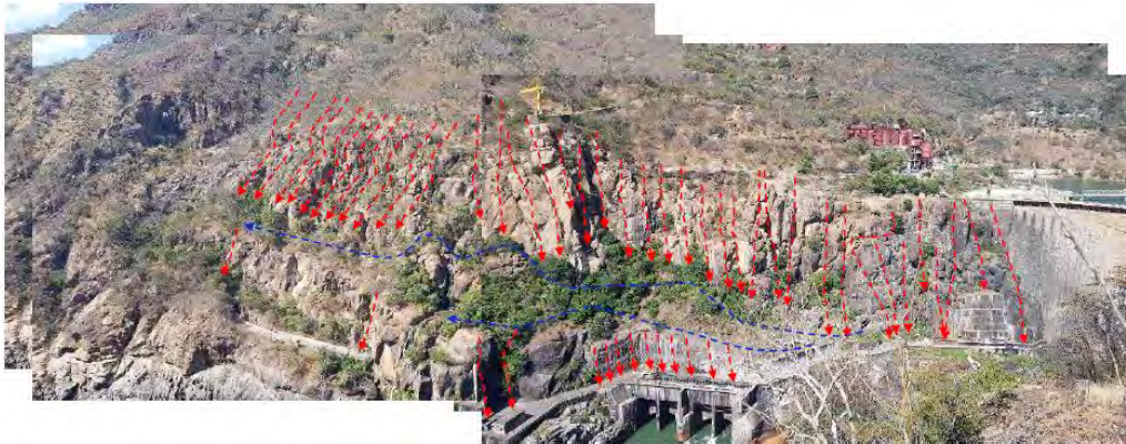
Evaluation of the trajectory of unstable elements and coverage of the terrain crossed. These trajectories were studied in the office on tracking software, but the observation and “feeling” in the field were also very important (presence of trees that can impact trajectories, small intermediate projections, etc.).
