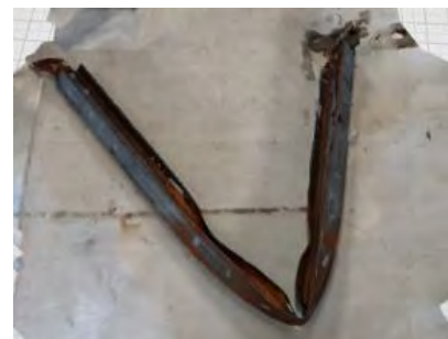
Figure 1(b). Deformed steel post
