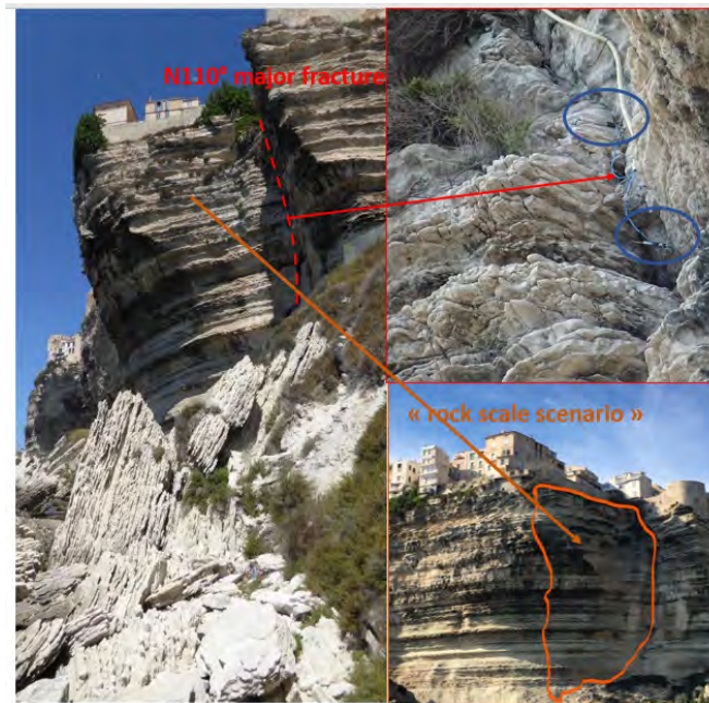
Figure 2. location of the two crack meters and “rock scale scenario”
