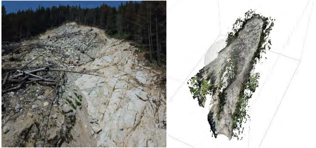
Figure 3. Left: Seabird Island landslide, view of the left flank and scarp area. Right: 3D model of the rock slide, produced with SfM photogrammetry from drone flights photographs.
