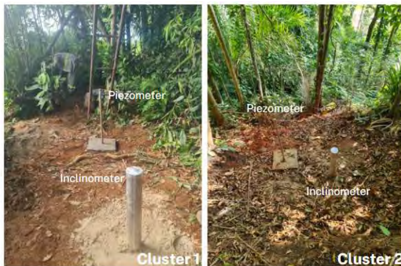
Figure 2 Piezometers and inclinometers installed in Cluster 1 (left) and in Cluster 2 (right).
