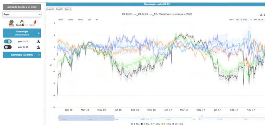
Figure 4 : Screenshot of the web portal Evorisk, visualizing the results of passive seismic monitoring at Gugla rock glacier.
