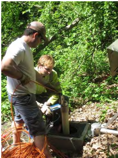
Figure 2. Inclinometer SC1: a- in situ measurements, b- cumulative horizontal displacements since 09/12/2009
