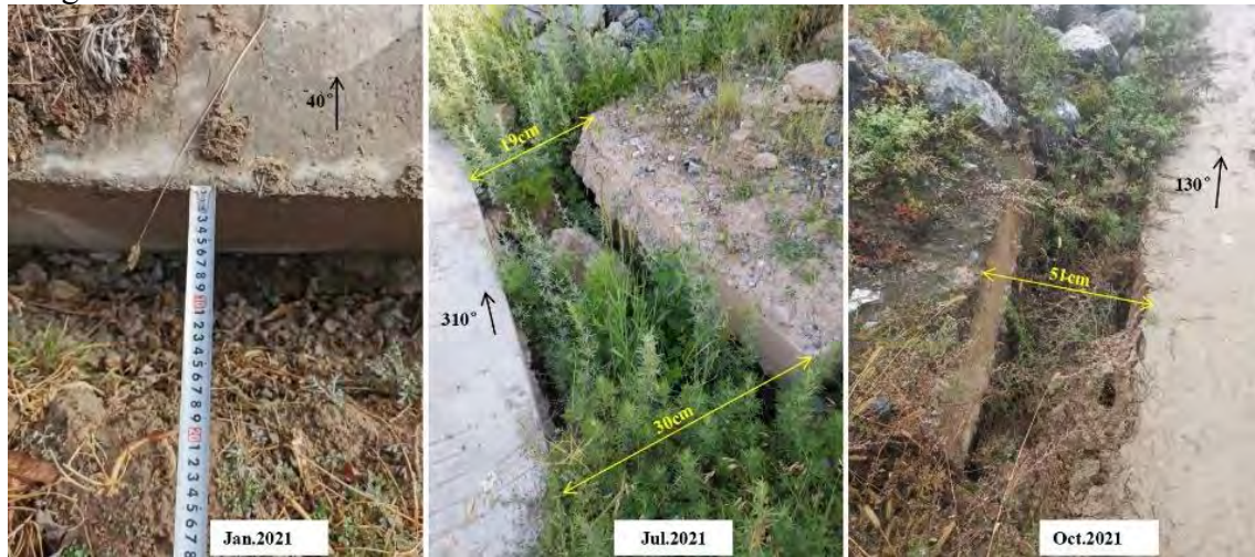
Figure 6. Continuous crack extension indicating landslide creep (Point d in Figure 2)
